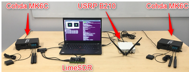
Fig. 4: Experimental testbed for targeted sidelink jamming.
