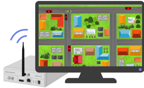
Fig. 2. A snapshot of the receiver’s (green vehicle’s) perspective in V2Verifier . Each nearby (red) vehicle’s location is updated with each message from that vehicle, and the validity of the most recent message is indicated by translucence of vehicles whose last message did not contain a valid signature.
